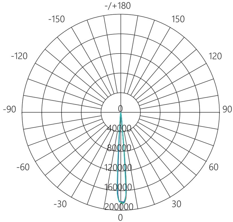
Small beam angle (beam angle): 8.1°
