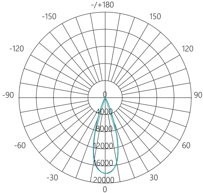
Widest beam angle (beam angle) :33.2°
